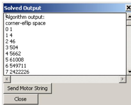
To actually move the real cube we click **Send Motor String**, and the string of commands is sent to the EB63 over the serial line COM2. The final result of the motion commands is as follows:
