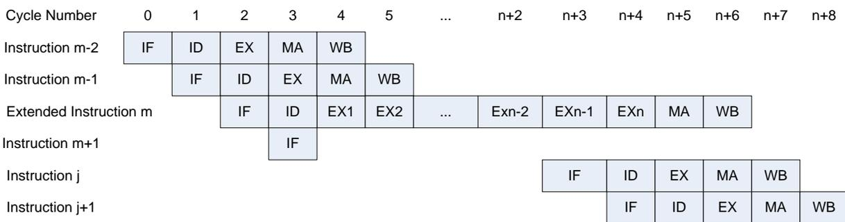
Figure 1: Scheduling of instructions through the eMIPS Pipeline with the extended instruction (Instruction  $m$ )
