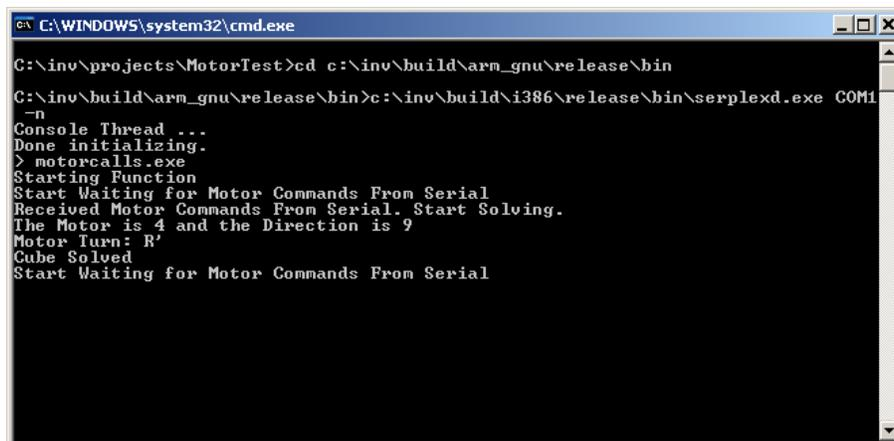
As shown above, in this case the program received a single command to move the **Right Motor** Counterclockwise 90 degrees. The encoding for “Motor Turn” is:
