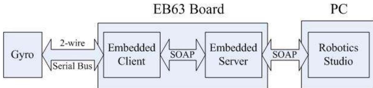
At the start, Embedded Client asks Embedded Server to create a web service for itself. This service is called ‘TEST’ and will serve to hold the gyro data. The SOAP messages exchanged are as follows.
