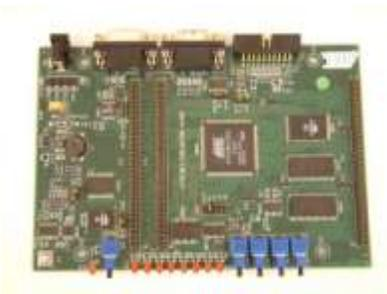
The microcontroller used in the demo is the Atmel EB63 Arm7 board, which runs at 25MHz. This board is loaded with the Microsoft Invisible Computing platform. Tasks include polling the gyro and managing the web services used to communicate with Robotics Studio. Because the board has no Ethernet port, the Ethernet packets generated by the network protocol are sent via a serial line to the PC and are then forwarded using a Virtual NIC driver.
