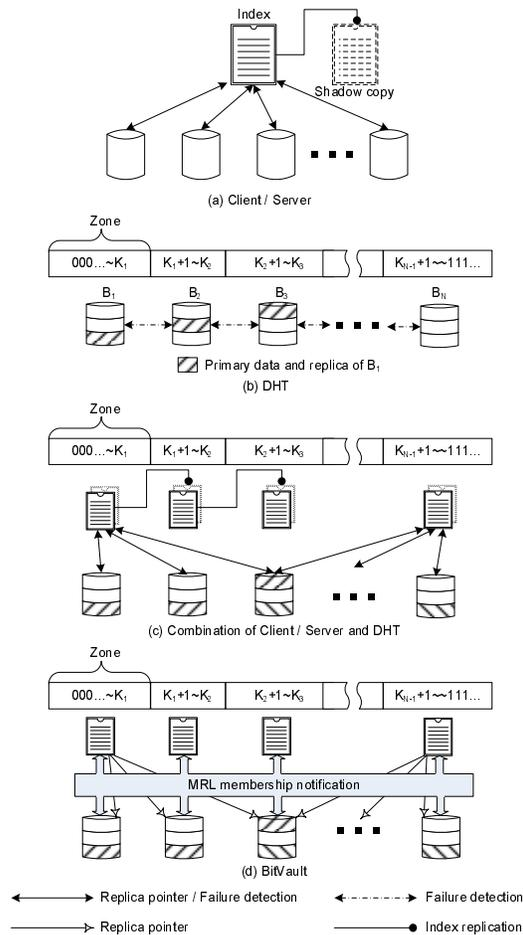
**Figure 1. Different architectures for a scalable brick-based system: (a) client-server; (b) DHT, (c) DHT + client-server and (d) DHT-based index partition, policy controlled object placement with a membership service.**
