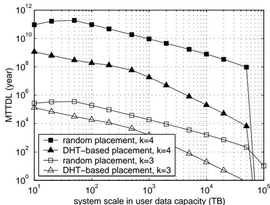
Figure 2. Analytical result on data reliability as measured by *MTTDL* (mean time to data loss) for various system scales, replication degrees, and placement schemes. The average object size in random placement is 10MB. Each brick has capacity of 100GB, with disk bandwidth 5MB/s. The network aggregated bandwidth for data repair is 3GB/s. Mean time to failure of each brick is 1000 days. Each brick fails independently with exponential distribution.
