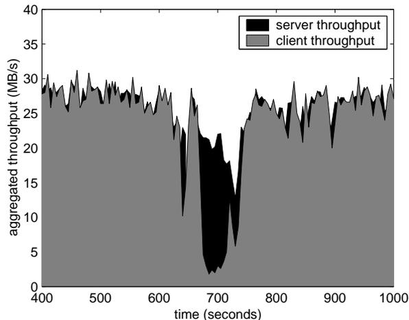
**Figure 10: performance under failure experiment.** Server throughput is normalized by 3. A failure is introduced around the 10<sup>th</sup> minute.
