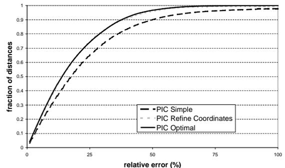
Fig. 7. Cumulative distribution of relative errors over random distances in GATech, using two algorithms to find close nodes.
