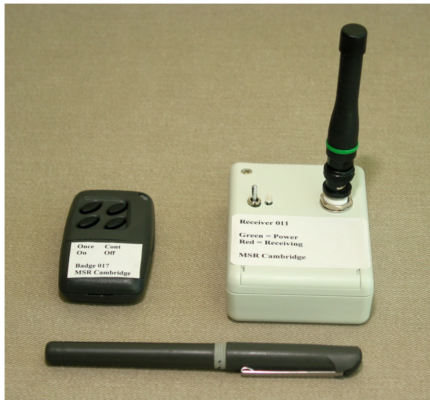
Fig. 1. The badge transmitter is on the left, with buttons for on, off, one-time transmit and periodic transmit. The receiver, on the right, is powered externally and connects to a PC via RS-232. The receiver measures the signal strength of transmissions from the badge. The pen is just a pen.
