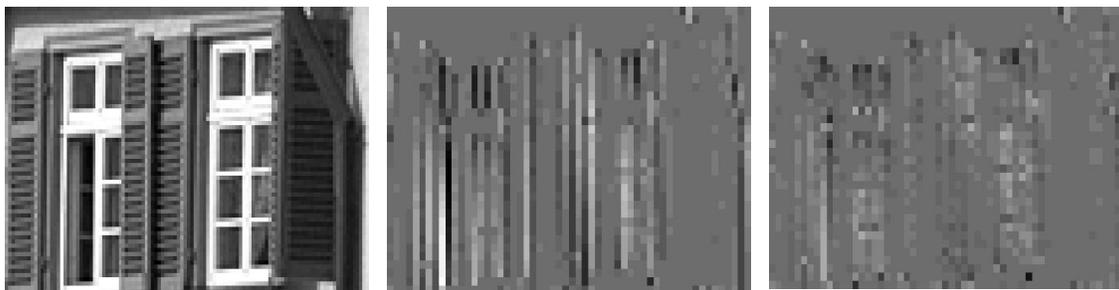
Figure 10: Example of prediction efficiency. Left: image section under test. Center: wavelet coefficients before prediction (amplitudes plotted as pixel intensities; zero is mid gray). Right: after prediction – note how the network is efficient in predicting edges.
