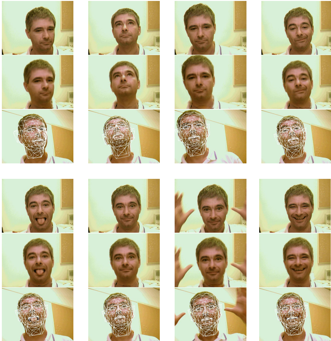
Figure 7: Sample results from the second test sequence. The upper and lower rows are the original stereo images, while the middle rows are the synthesized ones. The triangular face model is overlaid on the bottom images. From left to right and from top to bottom, the frame numbers are 159, 200, 400, 577, 617, 720, 743, and 830.
