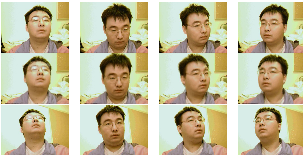
Figure 6: Sample results from the first test sequence. The top and bottom rows show the images from the top and bottom cameras. The middle row displays the synthesized images from a virtual camera located in the middle of the real cameras. The frame numbers from left to right are 108, 144, 167 and 191.
