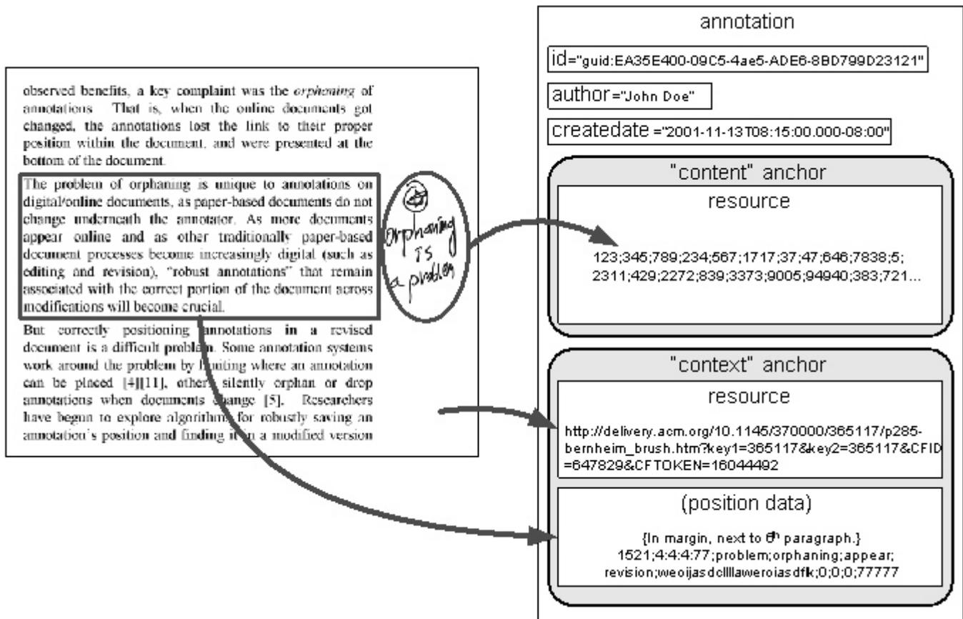
**Figure 1: Common Annotation Framework (CAF) logical model for a handwritten annotation on a text document. CAF annotations are self-contained and symmetrically structured to support a wide range of annotation functionality. The numbers in the "content" anchor represent digital ink coordinates.**
