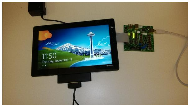
Figure 3: Windows RT 8.1 power profiling setup #2: Pre-instrumented to gather fine-grained power numbers for a smaller set of power rails including the CPU, GPU, Screen, WiFi, eMMC, and DRAM.
