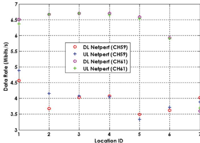
Figure 15: Throughput comparison between Channel 59 and Channel 61
