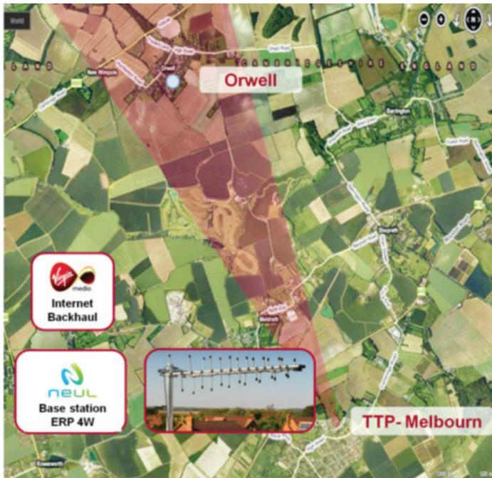
Figure 16: The TTP Base station providing broadband service to Orwell
