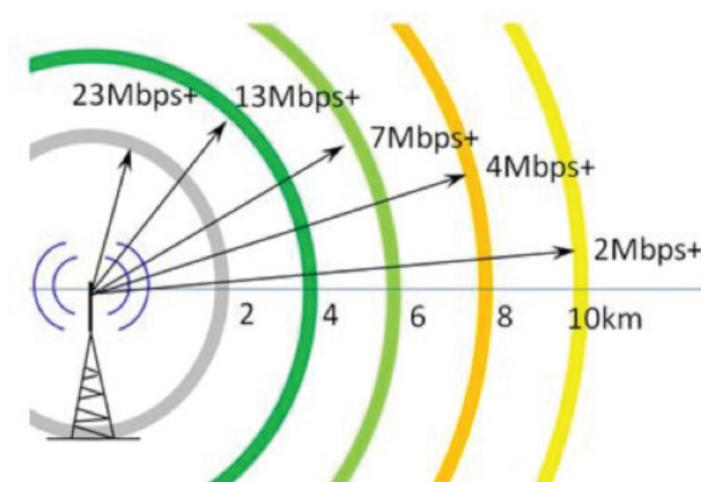
Figure 18: Analysis based on Shannon +3 dB margin and 65 % PHY>MAC> Network packet efficiency with 60/40 downlink vs uplink timings
