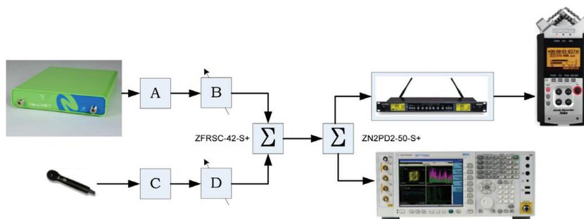
Figure 24: Radio Microphone Bench Test Configuration
