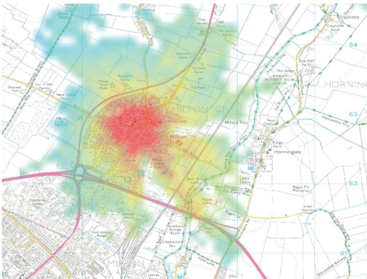
Figure 14: UKPM Coverage Prediction for CH 61 BS Coverage
