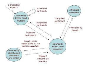
Figure 2. Object lifecycle for an arbitrary object o.
