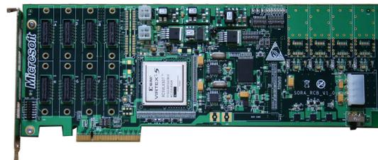
Figure 1: Sora radio control board.
