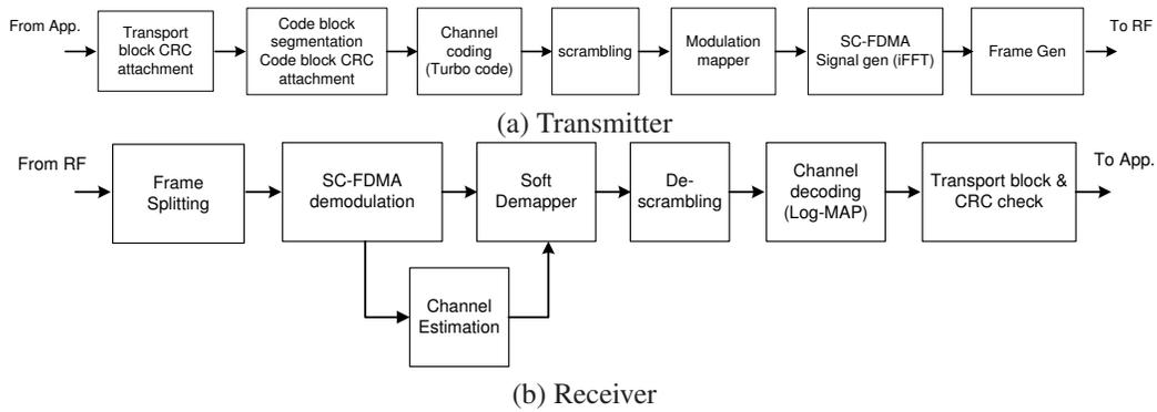
Figure 2: Illustration of LTE PUSCH transceiver.
