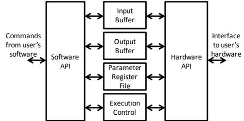
Figure 1. High-level relationship between the software & hardware APIs
