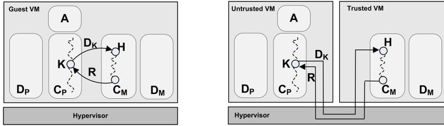
Figure 1: (a) In-VM and (b) Out-of-VM monitoring
