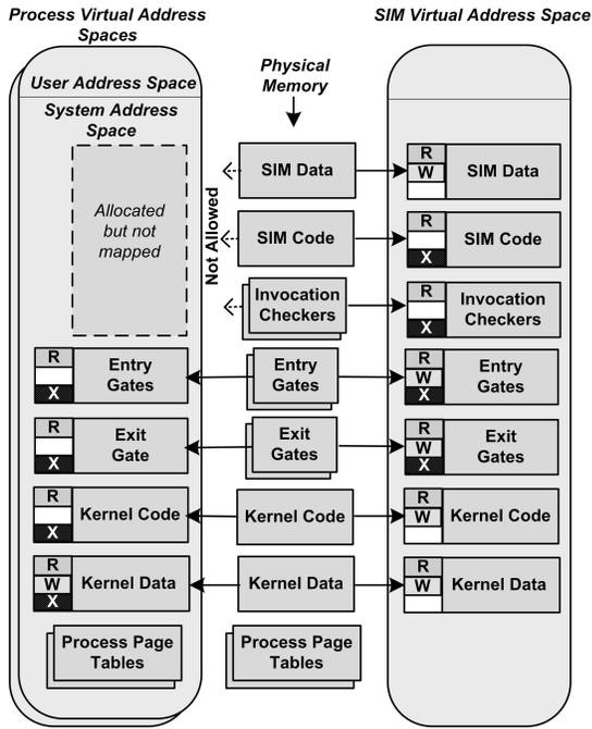
Figure 3: Virtual Memory Mapping of SIM approach.
