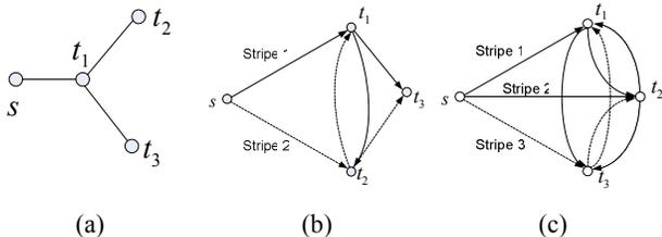
Figure 2 Prior one-to-many content distribution schemes: a) Scattercast/Overcast, b) SplitStream/CoopNet, c) FastReplica.
