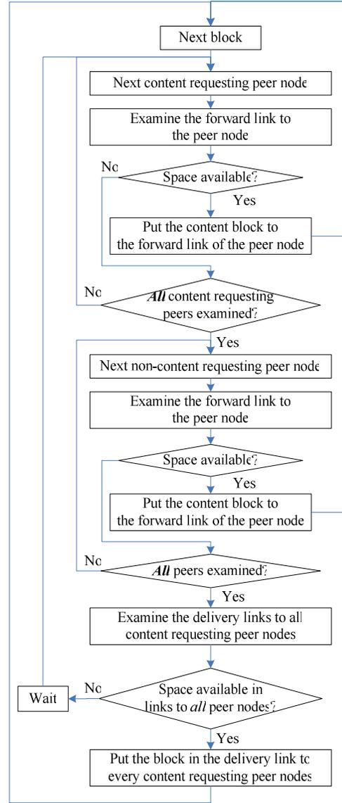
Figure 6 The operation flow of the source node.
