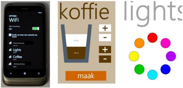
**Figure 2.** To access a SAWUI, a user chooses the appliance from the WiFi settings screen (left) of their phone. The SAWUI automatically appears with no further user input. We prototyped a SAWUI-controlled coffee machine (middle) and mood light (right). The phone’s language setting is used automatically. Cookies store personal settings persistently.
