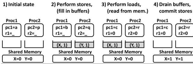
**Figure 1.** Snippet of Dekker’s mutual exclusion protocol (top). The sequence (bottom) is possible on most contemporary multiprocessors and shows how the protocol fails to achieve mutual exclusion on TSO.
