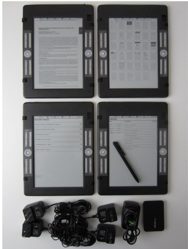
**Figure 1 - Full set of equipment (consisting of slates, stylus, Wi-Fi hotspot and power adapters) provided to participants. Slates above are showing the four UI views in the system (clockwise from top left: Page, Thumbnail, Library, Stack).**
