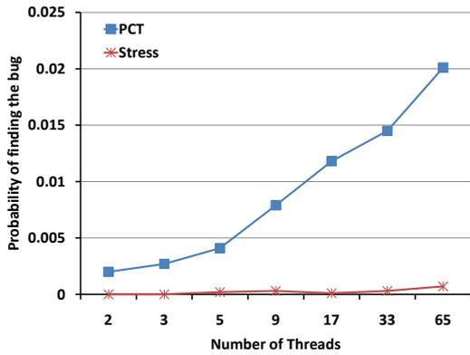
Figure 10: Probability of finding bugs with PCT and Stress with increase in threads and number of threads
