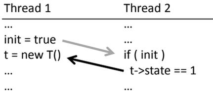
**Figure 4:** Although it may seem like one constraint (black arrow) is sufficient to find this bug, an extra constraint (gray arrow) is needed to ensure that thread 2 really executes the access of `t`. Thus, the depth of this bug is 2.
