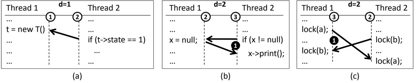
**Figure 6:** Illustration on how our randomized scheduler finds bugs of depth  $d$ , using the examples from Fig. 1. The scheduler assigns random initial thread priorities  $\{d, \dots, d + n - 1\}$  (white circles) and randomly places  $d - 1$  priority change points of values  $\{1, \dots, d - 1\}$  (black circles) into the execution. The bug is found if the scheduler happens to make the random choices shown above.
