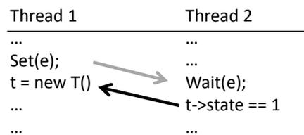
**Figure 3:** A variation of the example in Fig. 1(a). This bug requires Thread 1 to be preempted right after the instruction that sets the event  $e$ . Hence this bug has a *preemption bound* of 1 while the bug in Fig. 1(a) has a *preemption bound* of 0. Both bugs are of depth 1.
