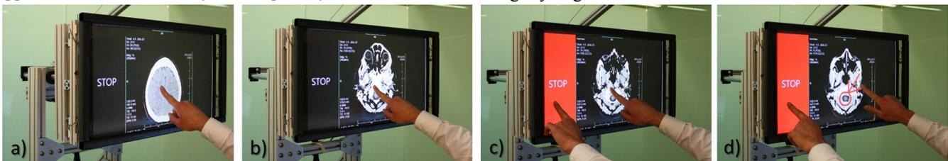
**Figure 9. Interacting with medical volumetric data. We used the MRI scans of the human brain in our application. Pushing the display back reveals different images of the scan dataset (a-b). The user can prevent the device from moving by touching on a stop button (c) and then annotating the current slice with their finger (d).**
