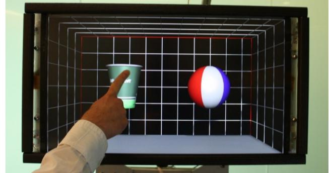
**Figure 8. 3D contour tracing application where the user feels the shape of the 3D object by tracing their finger along its surface. Note: stereo rendering is disabled for clarity.**
