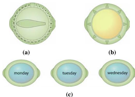
**Figure 4a.** Example of timer alert designed for days of month. The magnet is manually turned to set alert. **4b.** Glowing magnet designed to glow for 24 hours when moved on/attached to fridge surface. **4c.** Three of the possible seven magnets assigned to days of the week. If, for example, the ‘Monday’ magnet is moved on the fridge surface, it will glow on the upcoming Monday.
