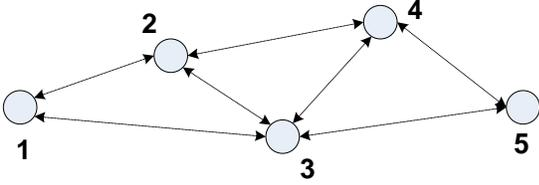
Fig. 2. Forwarding example. Lines connect nodes that can exchange packets. Opportunistic routing implies multiple-paths. Possible paths from 1 to 5 are for example  $(1, 2, 3, 4, 5)$ ,  $(1, 2, 3, 5)$ ,  $(1, 2, 4, 5)$ ,  $(1, 3, 4, 5)$ ,  $(1, 3, 5)$ . Path  $(1, 2, 1, 3, 5)$  is also possible but will be typically eliminated by a routing protocol due to suboptimality.
