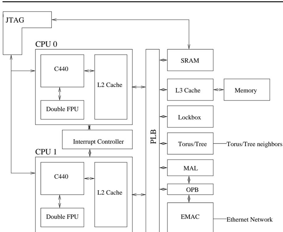
**Fig. 3.** The internals of a BlueGene/L node.
