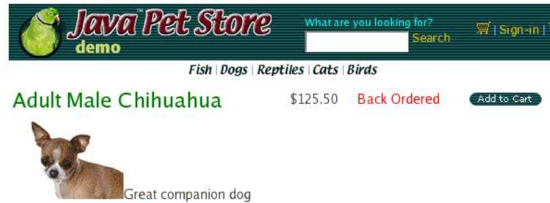
Figure 5.6: A masked failure in Petstore 1.1. During an Inventory database failure, Petstore 1.1 attempts to mask the problem, showing items as back-ordered, instead of displaying an error
