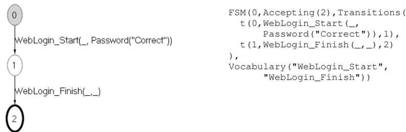
**Fig. 2.** A login scenario restricting the behaviour to only trying correct passwords.
