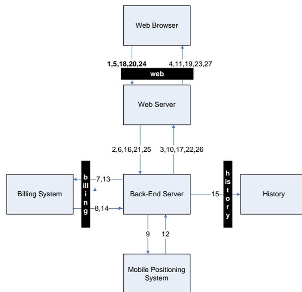
**Fig. 5.** Architecture of the WorkForce Management system.
