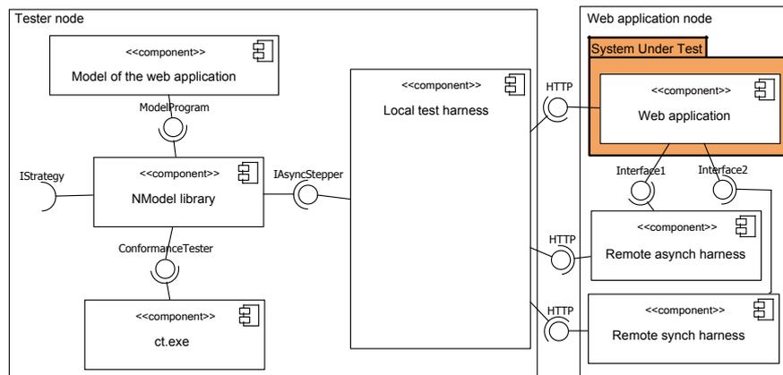
**Fig. 3.** A SysML component diagram of the setup of model-based testing of a web application.
