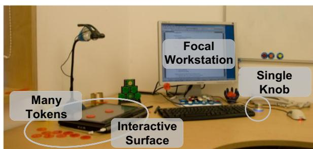
Figure 1. Structural design of TUI
