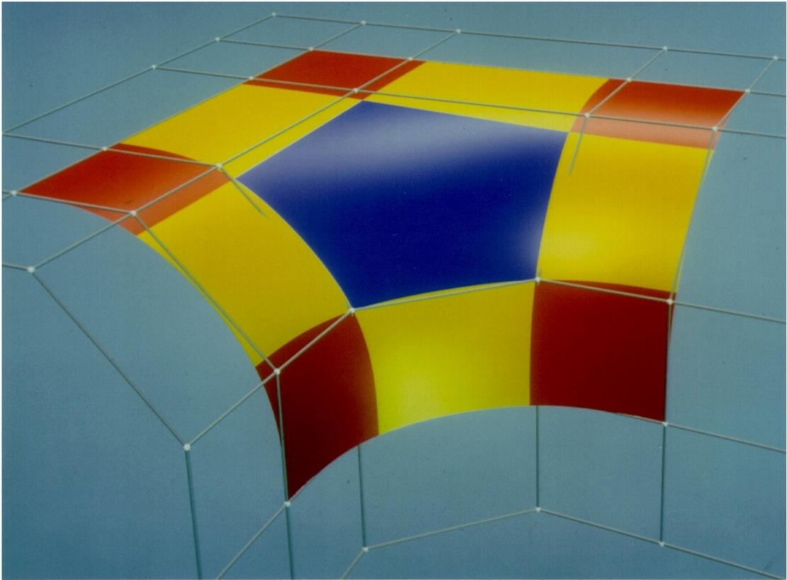
Figure 5.7: A 5-sided patch in an otherwise rectangular control mesh
