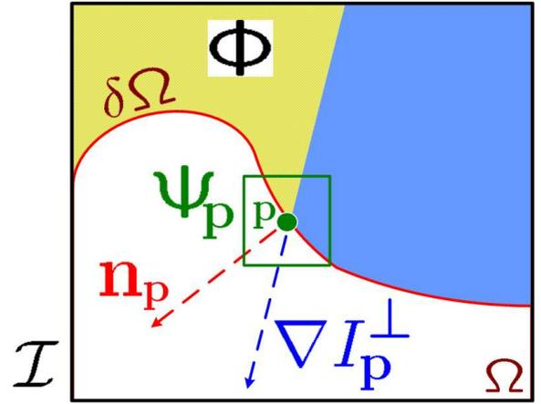
Fig. 5. **Notation diagram.** Given the patch  $\Psi_{\mathbf{p}}$ ,  $\mathbf{n}_{\mathbf{p}}$  is the normal to the contour  $\delta\Omega$  of the target region  $\Omega$  and  $\nabla I_{\mathbf{p}}^{\perp}$  is the isophote (direction and intensity) at point  $\mathbf{p}$ . The entire image is denoted with  $\mathcal{I}$ .
