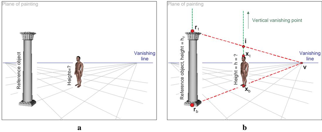
**Figure 6:** *Measuring heights in paintings. (a) We wish to compute the height of the human figure relative to the height of the column. The vanishing line of the image is supposed to have been computed (shown in blue). (b) The ratio between the height of the man and that of the column is given by  $\frac{h}{h_r} = d(\mathbf{x}_t, \mathbf{x}_b)/d(\mathbf{i}, \mathbf{x}_b)$ . See text for details.*
