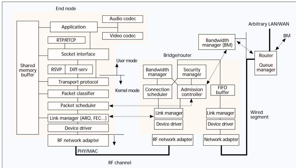
■ Figure 9. Software architecture for packet flow from a wireless node to a wired segment.
