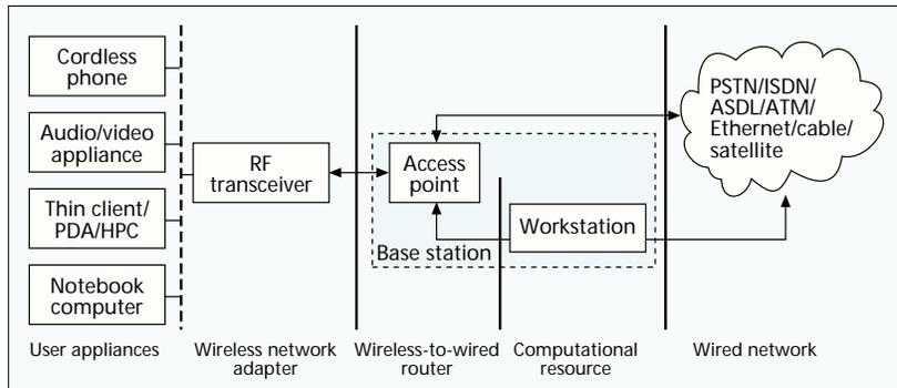
■ Figure 2. Reference architecture for a managed wireless network.
