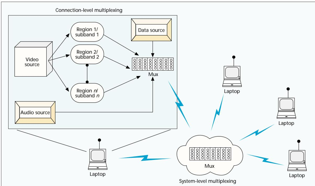
■ **Figure 5.** Combining connection-level and system-level statistical multiplexing.
