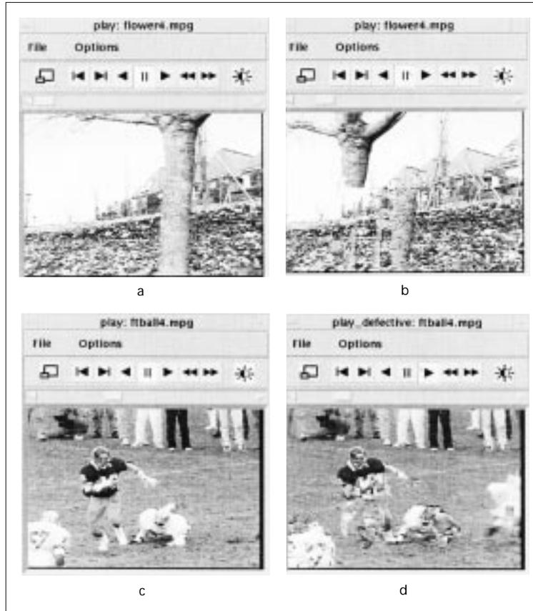
Figure 1. The effect of temporal and spatial error propagation in current ISO and ITU video codecs: a) frame #16; b) frame #31; c) original; d) with spatial error propagation.
