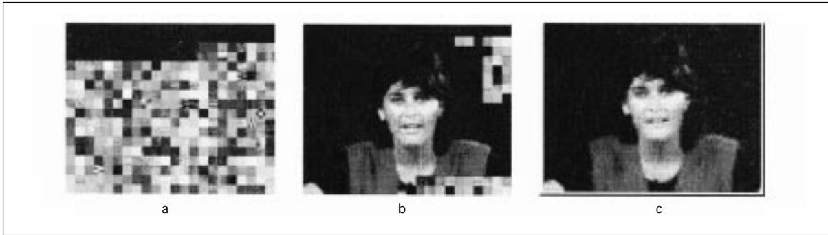
■ **Figure 4.** Alleviating error propagation with spatial and frequency decomposition: a) bitstream corruption of the Miss America sequence in ITU's H.263; b) after region segmentation; c) after region segmentation, frequency segmentation, and prioritized transmission (PSNR: 3.2.34 dB).
