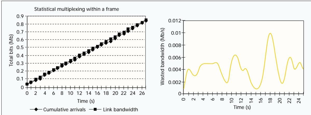
■ Figure 6. Intraframe statistical multiplexing for a region-segmented video codec.
