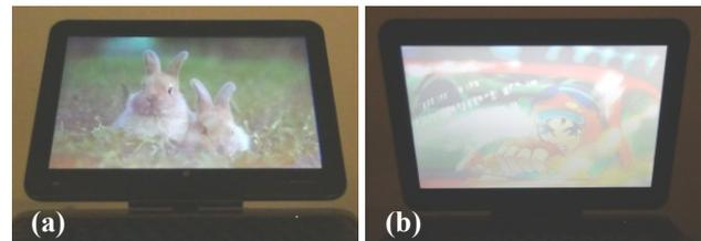
**Figure 1. A common laptop screen based on TN LCD showing two images concurrently for different viewing angles. (a) Bottom view. (b) Top view.**
