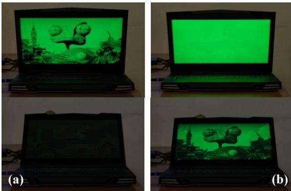
Figure 5. Image rendered with continuous brightness range (G channel only). (a) Image shown at +25° and hidden at -25°. (b) Image hidden at +25° and shown at -25°.
