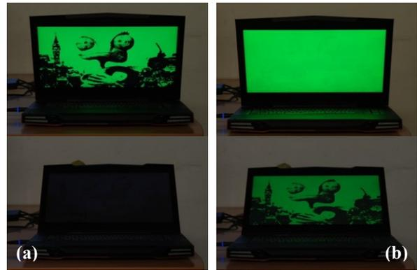
**Figure 4. Binary image. (a) Image shown at  $+25^\circ$  and hidden at  $-25^\circ$ . (b) Image hidden at  $+25^\circ$  and shown at  $-25^\circ$ .**
