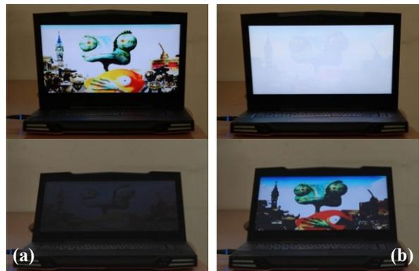
Figure 6. 8-color image with dithering. (a) Image shown at +25°, hidden at -25°. (b) Image hidden at +25°, shown at -25°.
