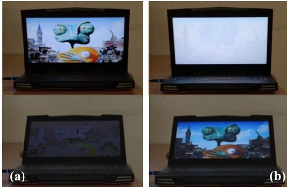
Figure 7. “Full-Color” image. (a) Image shown at +25° and hidden at -25°. (b) Image hidden at +25° and shown at -25°.
