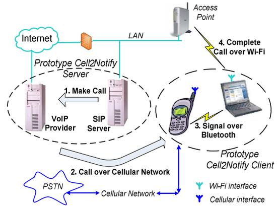
**Figure 5:** Our prototype implementation of Cell2Notify. We implement the Cell2Notify server as a combination of a commonly available SIP Proxy and an Internet-based VoIP gateway. We emulate a smartphone using a combination of a cellphone that communicates with a Wi-Fi equipped laptop using Bluetooth.
