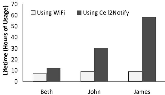
**Figure 8:** Energy consumption of a Cingular 2125 with and without Cell2Notify for three users. We assume that the user does not use the smartphone for any other purpose, but only for making and receiving VoIP calls.
