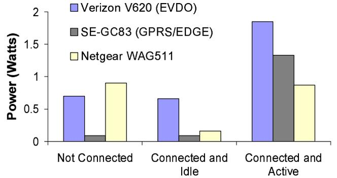
**Figure 2:** Power measurements of 1xEVDO, GPRS/EDGE and Wi-Fi interfaces for different scenarios. The “Connected and Active” measurements show the power when transmitting 32 Kbps of VoIP traffic over UDP. Note that when active, VoIP over Wi-Fi consumes the least amount of battery power.
