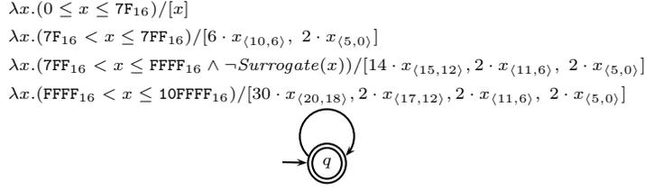
**Fig. 1.** SFT *EncUTF8*: UTF8 encoder for valid Unicode code points;  $x_{(h,l)}$  extracts bits from  $h$  to  $l$  from  $x$ , e.g.,  $8_{(3,2)} = 2$ ; *Surrogate*  $\stackrel{\text{def}}{=} \lambda x.D800_{16} \leq x \leq DFFF_{16}$ , surrogates are not valid code points;  $x \cdot y$  denotes bit-append, e.g.,  $6 \cdot x_{(10,6)} = C0_{16} + x_{(10,6)}$ .
