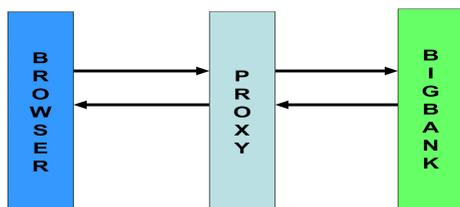
**Figure 1: The basic design. All traffic from the browser on the untrusted machine flows through a MITM proxy. The user enters the password using an obscuring method; it is unobscured at the proxy. Once login is established the proxy reverts to a passive rôle.**
