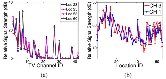
Figure 5: (a) Location 23, 25, 53 and 60 receive close signal strengths from many TV channels. Each line represents the relative signal strengths received at an indoor location for 42 channels. We observe strong location correlation. (b) CH 1 and 3 exhibit very close signal strengths at different indoor locations. Each line represents the relative signal strengths for a channel at 65 indoor locations. We observe strong channel correlation.
