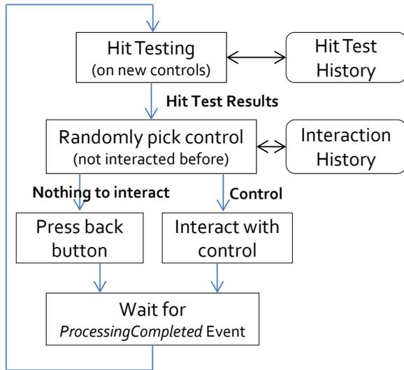
Figure 12: UI automator flow.
