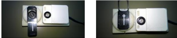
**Figure 2:** An initial hardware prototype of courteous glass that uses a FIR imager to implement the courtesy protocol shown in Figure 1. The RGB camera can be covered up (as shown in the right picture) when the FIR imager detects new people in FoV who have not consented for recording yet.
