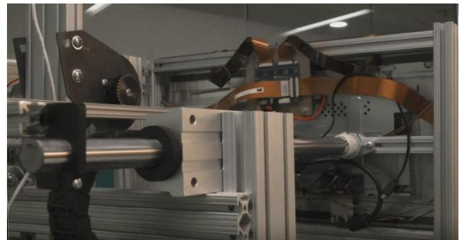
Figure 3: The 1D Robot Actuation image of the back side of our device showing the rack and pinion gear and the completely supported 3D touchscreen up front.
