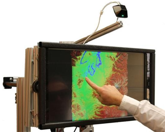
Figure 1: TouchMover 2.0 co-locates immersive 3D stereo visualization, direct touch and touch force sensing with a robotically actuated display and a vibrotactile screen.
