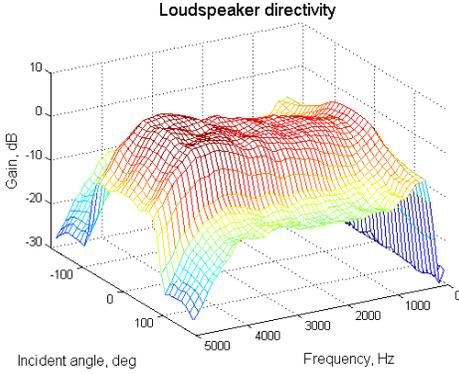
**Figure 2.** Loudspeaker magnitude response.
