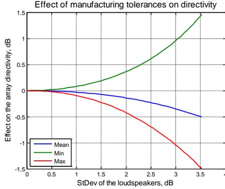
**Figure 1.** Effect of manufacturing tolerances on the loudspeaker array directivity.
