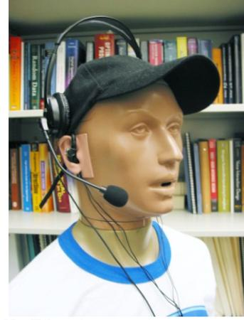
Figure 2. HATS with microphone array and headset.
