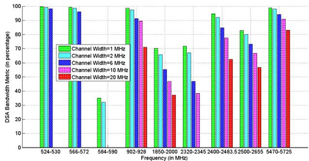
Fig. 6. DSA Bandwidth Metric (in percentage) remains same or decreases for different spectrum bands as channel width increases. Note that DSA Bandwidth Metric (y-axis) is plotted as a percentage of the absolute bandwidth available in the band, i.e. 50% availability in 150 MHz provides more bandwidth than 100% availability in a 6 MHz band.
