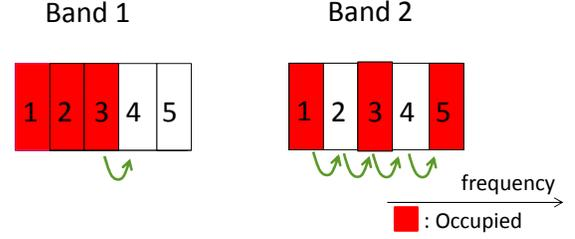
Fig. 3. DSA bandwidth metric for Band 1 is higher than Band 2 because a contiguous spectrum chunk is available to white-space device in Band 1. Each transition from or to an unused spectrum chunk (green arrows) is penalized by guard bands.
