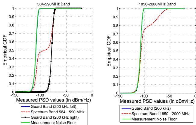
Fig. 5. Cumulative distribution function of measured PSD values in (a) (left) TV channel 584–590 MHz (b) (right) Advanced wireless services 2 (AWS2) band 1850–2000 MHz. Note that the measurement noise floor (green) and guard band (blue) curves overlap.
