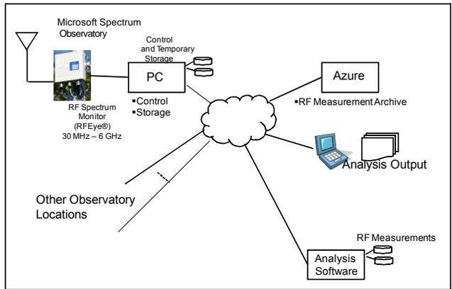
Fig. 1. Setup of the Microsoft Spectrum Observatory. Power spectral density measurements are collected in 30 MHz–6 GHz by a wideband antenna and RFEye receiver device. The data is stored in the cloud and selectively retrieved by analysis software to obtain DSA goodness metric etc.
