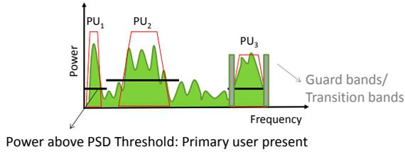
Fig. 2. Plot of collected PSD values with frequency (x-axis). The collected PSD values correspond to primary user’s transmission or noise. A guard band can be used to determine the licensed user’s noise floor. PSD Threshold is chosen such the PSD values below the threshold indicate unused spectrum available to a white-space device.
