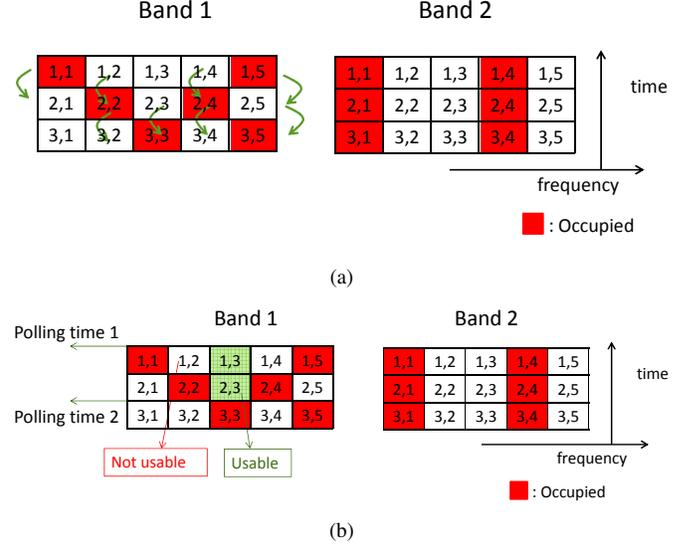
Fig. 4. DSA detectability metric is higher for Band 2 because the contiguous spectrum chunks have fewer transitions and thus lower overhead in detection and handshake as shown for (a) Oracle based or sensing based DSA techniques and (b) Geo-location based DSA techniques.
