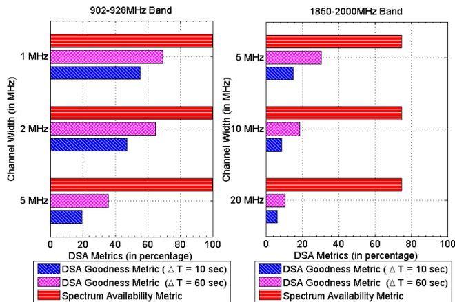
Fig. 8. Comparison of Spectrum Availability Metric and DSA Goodness Metric (in percentage) for different channel widths and transmission time interval  $\Delta T$  in, (a) (left) ISM band 902–928 MHz and (b) (right) Advanced wireless services 2 (AWS2) band 1850–2000 MHz. DSA goodness metric decreases as both channel width and  $\Delta T$  increases. Note that DSA metrics (x-axis) are plotted as a percentage of the absolute bandwidth available in the band.
