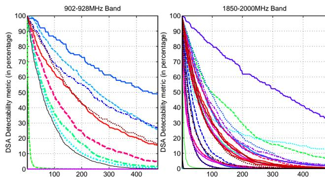
Fig. 7. DSA Detectability Metric (in percentage) for different contiguous chunks decreases as transmission time duration  $\Delta T$  increases for (a) (left) ISM band 902–928 MHz with channel width = 2 MHz, (b) (right) Advanced wireless services 2 (AWS2) band 1850–2000 MHz with channel width = 5 MHz. Note that the rate of decrease can vary widely for different contiguous chunks in the same band.
