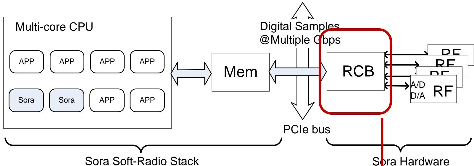
PCIe-based High-speed Interface card
