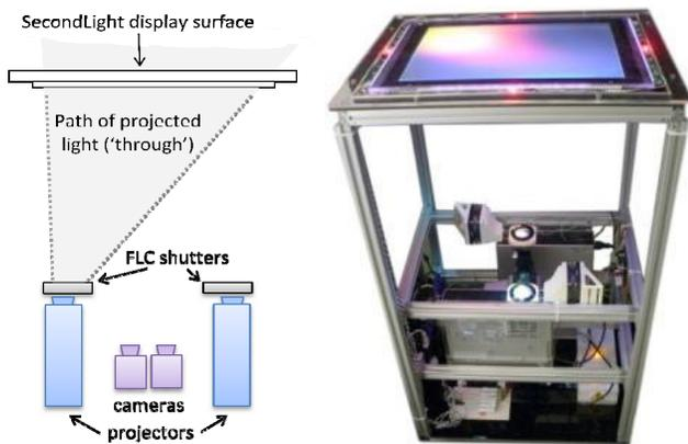
Figure 10: The layout of the main SecondLight components. On the left we show a cross-section through the side of the unit (this is during the 'through' phase when the second projector is active and light from the on surface projector is blocked). The far left is the front of the unit and thus the through projection is angled away from the user. On the right is a photo of the unit taken from the front.
