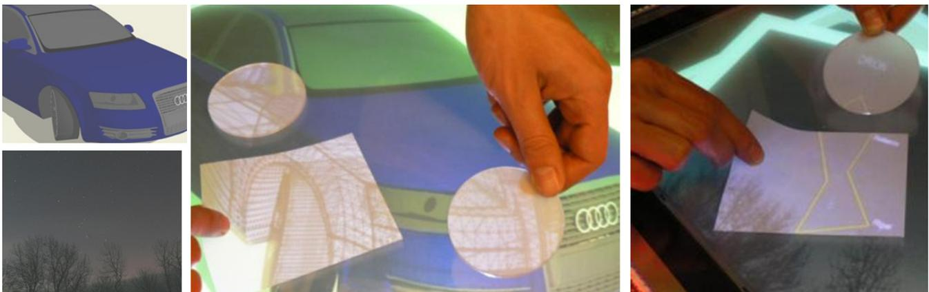
Figure 4: Creating tangible layering effects is extremely simple with SecondLight. A translucent sheet of diffuse film is placed above an image of a car to reveal its inner workings (middle) or above the night sky to reveal the constellations (right). Plain images are shown on left. Circular acrylic discs with diffuse topsides can be used to create a magic lens effect. Note how the magic lens image is maintained even if the disc is lifted well away from the surface.
