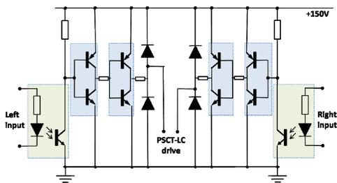
Figure 9: The PSCT-LC H-bridge driver circuit.
