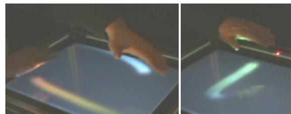
Figure 7: SecondLight allows gesture-based interactions with the primary surface from greater distances than many back projected systems (left).
