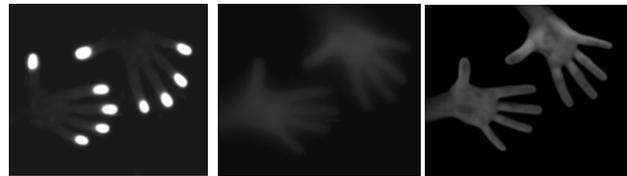
Figure 12: two hands imaged using FTIR (left) and diffuse illumination with the PSCT in diffuse (middle) and clear states (right)
