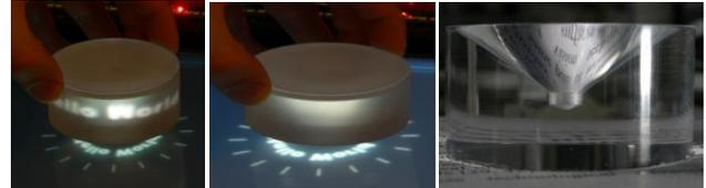
Figure 6: The ability to shine light through the display, gives rise to other novel tangible object designs. In this example, we demonstrate an object that uses internal prisms to project the incoming light onto its sides. The prism inside the object is shown right. The effect of the prism on the projection is shown left. The middle image shows the screen in a non-switching diffuse state – illustrating the behavior of a typical projection screen.
