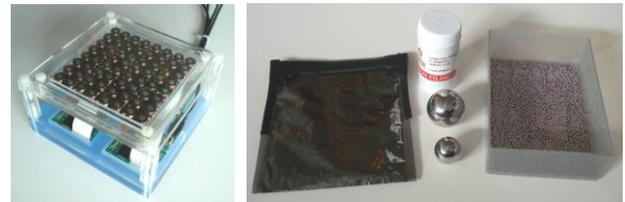
Figure 1: (left) hardware prototype which can sense ferrous objects such as (right) ferrofluid bladder, iron filings, large ball bearings and a box of small (2mm) ball bearings.
