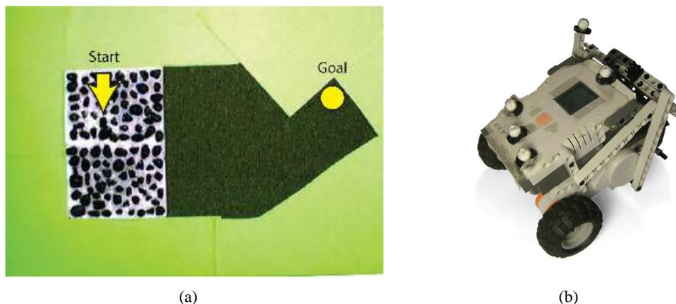
Figure 6: (a) Image of the environment. The start location and orientation is marked with an arrow. The goal location is indicated by the circle. (b) LEGO<sup>®</sup> robot.
