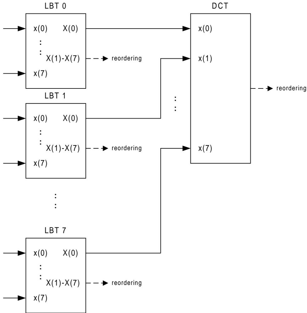
**Figure 3.** Six-level multiresolution decomposition (hierarchical transform) used in PTC. The DC coefficients of every eight LBT blocks are combined for the next transform stage. The DCT outputs are then reordered again to form the next three levels of the multiresolution decomposition.
