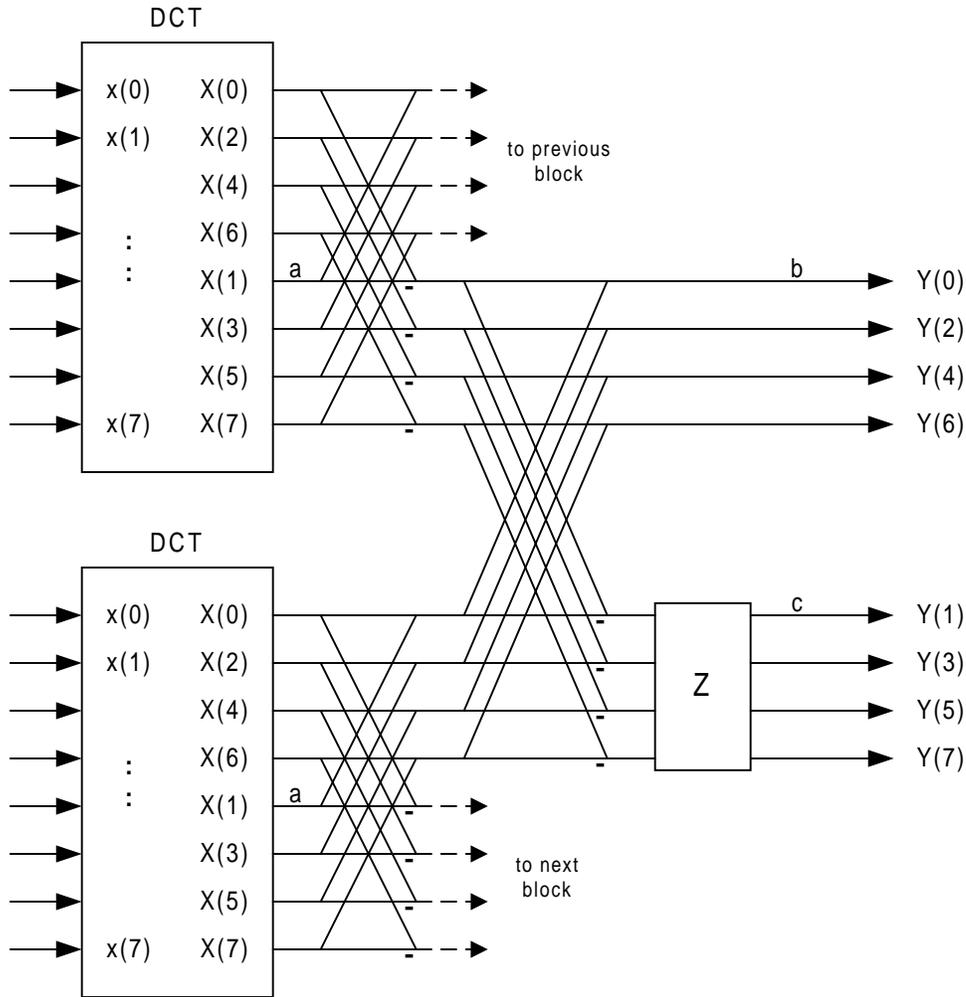
**Figure 1.** Flowgraph of the lapped biorthogonal transform.  $Z$  is a  $4 \times 4$  orthogonal matrix, as described in [11]. The scale factors  $\{a, b, c\}$  control the shape of the basis functions. The inverse LBT is obtained with the same flowgraph, with processing from right to left and  $\{a, b, c\}$  replaced by  $\{1/a, 1/b, 1/c\}$ .
