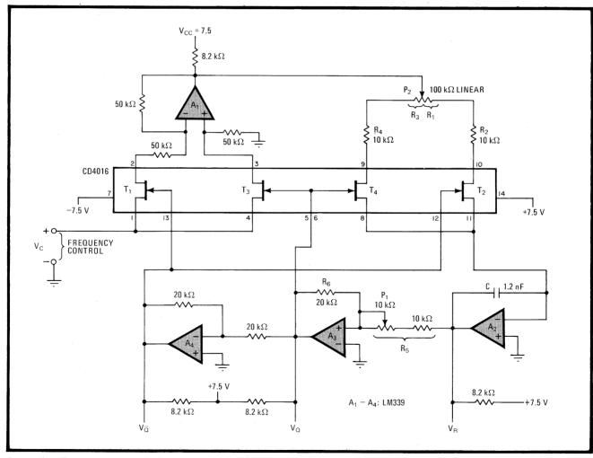
**Separation.** Transmission gates  $T_1 - T_4$  separate the portion of the ramp generator that determines the frequency from the circuitry that sets the charge and discharge times of its integrator, so that the up/down slope ratio and frequency can be independently selected. The inexpensive circuit, which costs less than \$10 and works in the audio range, is a useful timbre control in music synthesizers.
