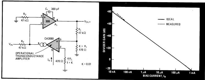
**Inverse.** A basic two-chip multiplier is easily transformed into a two-quadrant divider by the appropriate feedback. This scheme is simplier, no less accurate, and less costly than those using log and antilog converters. Circuit linearity extends to five decades of control current, I<sub>B</sub>. Except for the most critical applications, temperature compensation is not required.
