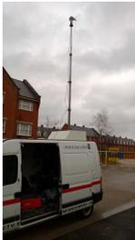
Figure 7: Van with 10m mast
