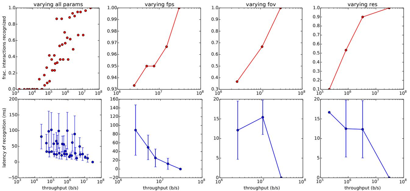
**Figure 1: Face recognition performance in fraction of interactions recognized (top) and detection latency (bottom) against throughput (X axis), while varying (a) all parameters, (b) frames per second, (c) field of view, or (d) resolution.**
