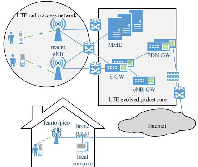
**Figure 2: Simplified depiction of the LTE cellular architecture. MME = Mobility Management Entity; PDN-GW = Packet Data Network Gateway; S-GW = Serving Gateway; eNB = E-UTRAN Node B.**
