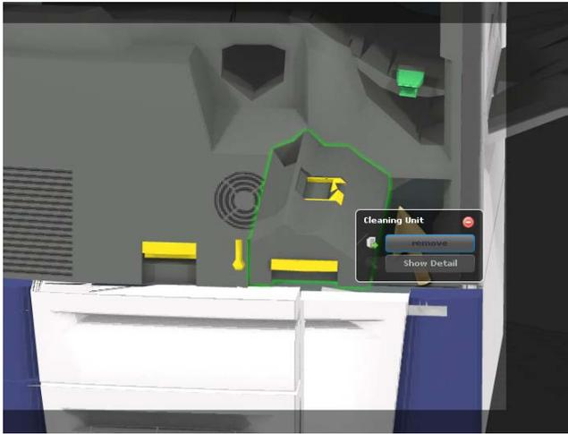
**Figure 7. Troubleshooter can ask to show how to remove the cleaning unit using the contextual menu popping up on top of the cleaning unit 3D model.**
